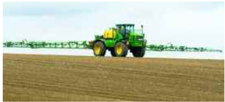
Topography can have an influence on boom height and stability, both factors influencing spray drift.
