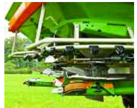
The Argus system checks the spread fan and automatically regulates the lateral distribution.
