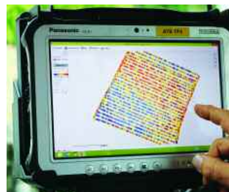
The service maps the unique radioactive signature emitted by the soil at 800 points/ha that’s influenced by its nutrient and mineral content.
