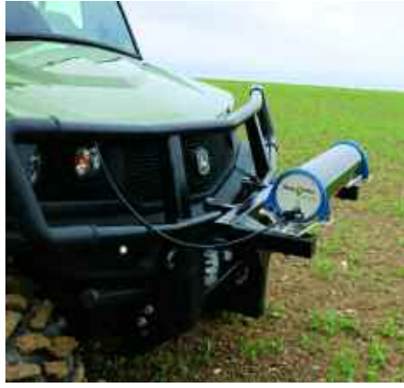
The scanner is a gamma ray spectrometer, mounted on a UTV, that passes no more than 1m above the ground.
