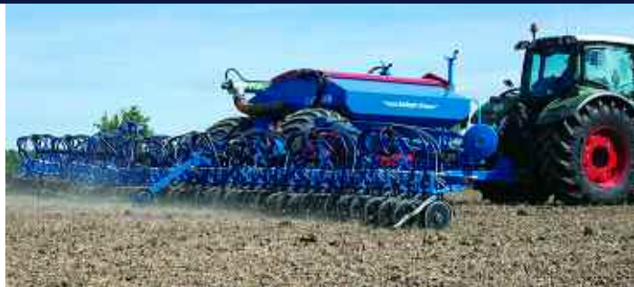
Lemken's Solitair 12 unit comes in working widths of 8-12m with an approximate hopper capacity of 5800 litres.
