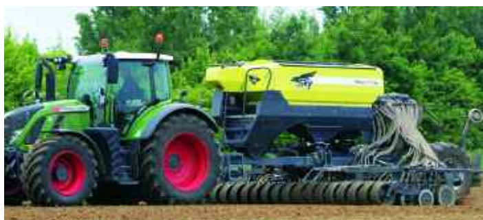
The Sky Easy drill can work direct into a cover or stubble, as well as into a cultivated field.
