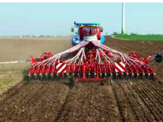
Pöttinger's Terrasem has a two-gang disc harrow with smooth or scalloped discs.
