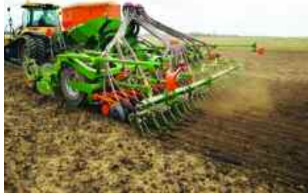
The Cirrus can prepare the seedbed and seed all in one pass with its two-row cultivation disc segment.
