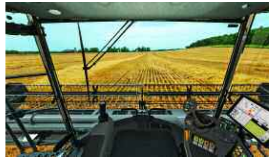
The Ideal 10 will be the first standard combine in Europe to be operated entirely without a steering wheel, claims Fendt.
