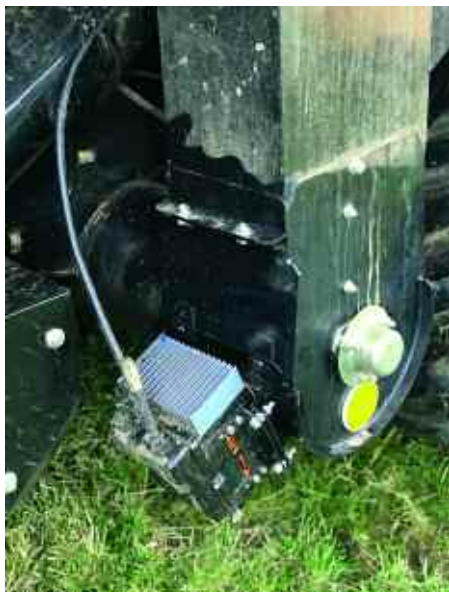
New Holland are experimenting with the use of an NIR as a means of early crop quality detection.
