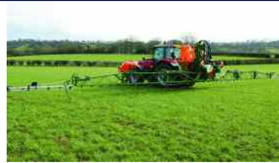
A move up to 24m wide booms from 20m was the main driver for change, bringing with it the latest spraying technology, including auto-levelling.
