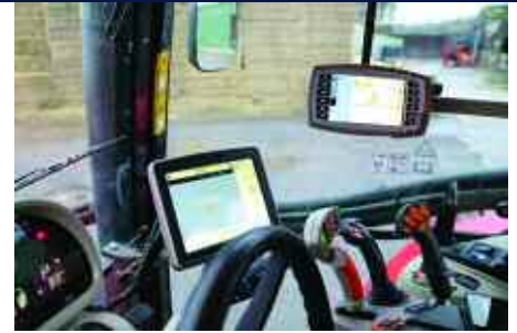
Massey Ferguson's Datatronic 4 terminal (right) runs the sprayer via ISOBUS, while The John Deere GreenStar looks after steering, mapping and section control.
