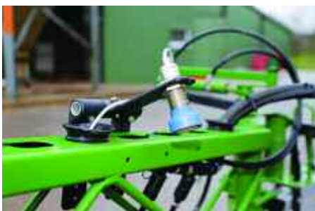
Sensors on the boom, supplied with Amazone's DistanceControl system, maintain the correct boom height.
