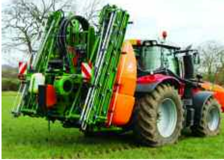
The 24m wide, rear-mounted booms can operate independently, are equipped with auto-levelling and fold to 2.4m wide for transport.
