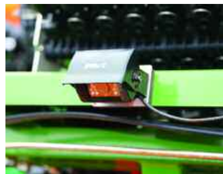
Alister Henson fitted this rear-view camera to help when reversing into corners and improve safety on the road.
