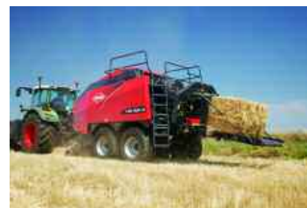
The recently introduced Kuhn LSB 1290 iD baler uses a two-part plunger to compress the bale in two stages, which increases the density by up to 25%.
