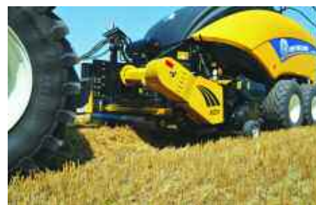
The New Holland TwinCutter option fits ahead of the pick-up and produces a finer straw chop using a rotor fitted with 44 knives and two rows of counter knives.
