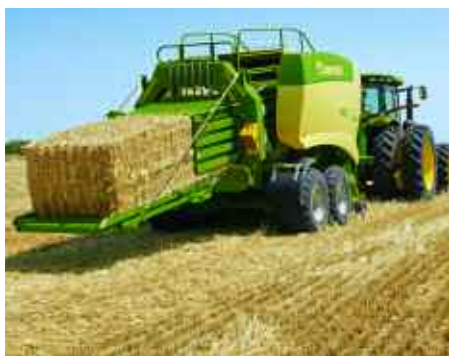
The Krone BIG Pack HDP system increases bale density by up to 25% and the machines are available in high speed version.
