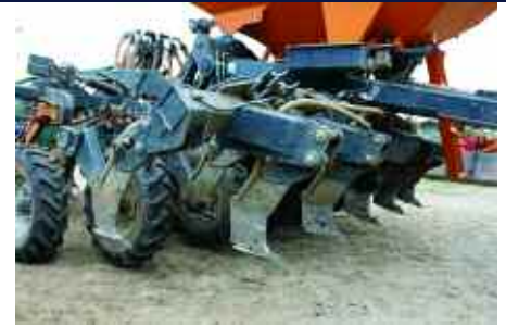
The cultivation leg itself is heavy duty and has a winged foot that loosens the ground and pulls up fresh earth for the seed to be planted in.
