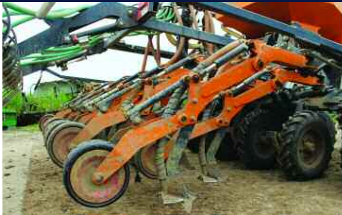
The coulters are mounted on a horizontal pivot so that the seed gets placed in the centre of the tilled strip.
