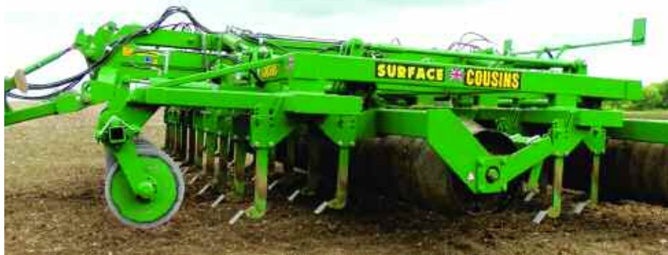
Dick Neale developed the Surface cultivator with Cousins specifically to create ideal conditions for germination and work at exactly 50mm depth.
