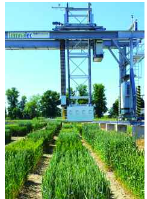
Much of the BBSRC-funded work at Rothamsted revolves around pre-breeding research, such as using its Field Scanalyzer, installed in 2014 to capture deep phenotyping data from crops and other plants growing in a real field environment.
