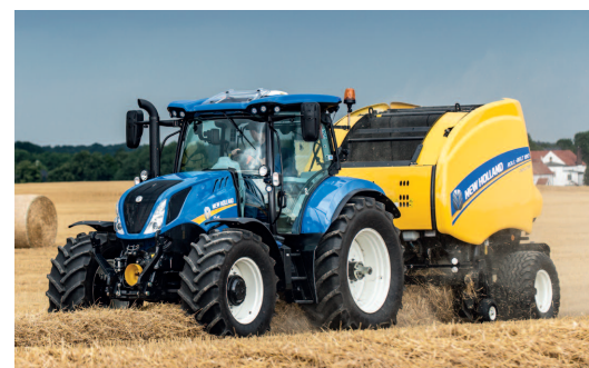
New Holland now fits 4.5 litre, four cylinder engines in all but the largest model in its latest T6 range of mid-power tractors.
