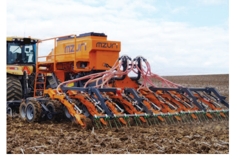
Mzuri's Pro-Til Select 6T is now fitted with the latest design spring-loaded pivoting discs that provide better straw clearance.
