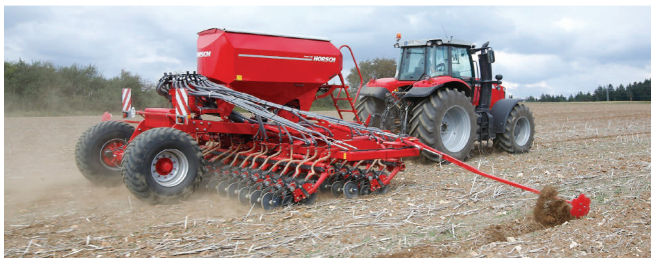
The Horsch Avatar SD is the first direct drill from the company and uses a straight disc to cut through trash followed by an angled opener disc and seed couler.
