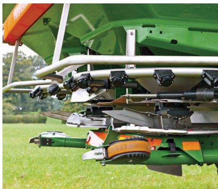
The Argus Twin system for the Amazone ZA-TS spreader uses radar sensors to monitor the application rate and distribution.
