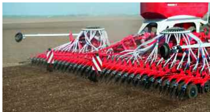
On the C8, there are 64 drill coulters, each mounted on an independent parallelogram which means they can follow the ground contours.
