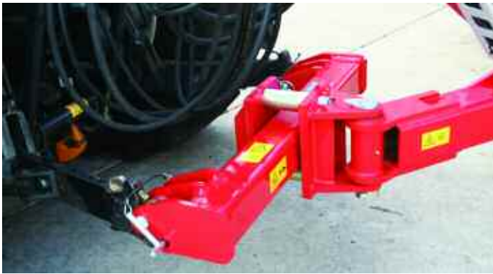
The linkage yoke means tight turns can be made on the headland without fear of scuffing.
