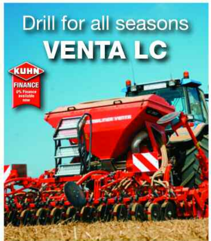
The linkage yoke means tight turns can be made on the headland without fear of scuffing.
