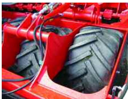
The central press wheels act as a combined packer and wheel unit, forming the centre of the drill.
