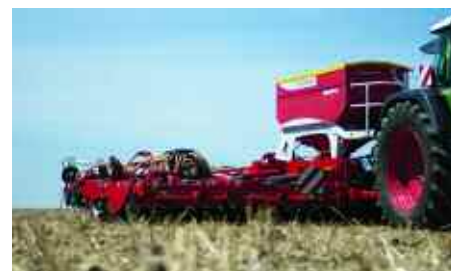
Although Stephen Craggs uses his C8 on ploughed ground, the drill can operate on worked stubbles, with the discs designed to handle a lot of trash.
