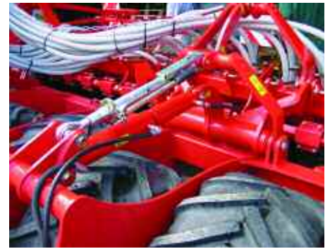
Coulter depth is adjusted via a central point, however pressure is hydraulically adjusted from the cab.
