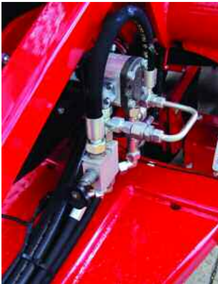
The high-volume hydraulic fan drive means there's a lot of air moving seed but at low velocity.
