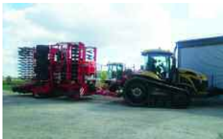
The drill folds to 3m for transport and can be specced with either hydraulic or air brakes.
