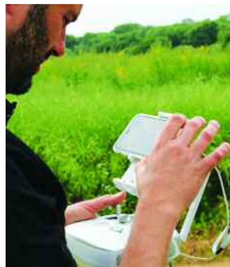
App-based software running on your smartphone or tablet usually controls the UAV.
