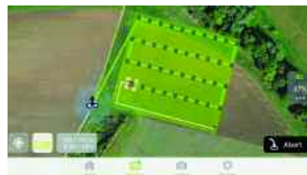
In survey mode, the drone completes a pre-planned mission which triggers the camera at pre-defined waypoints.
