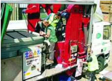
The pre-cleaner sieves the seed, and then it's gravity separated by weight, removing weed seeds in the process.
