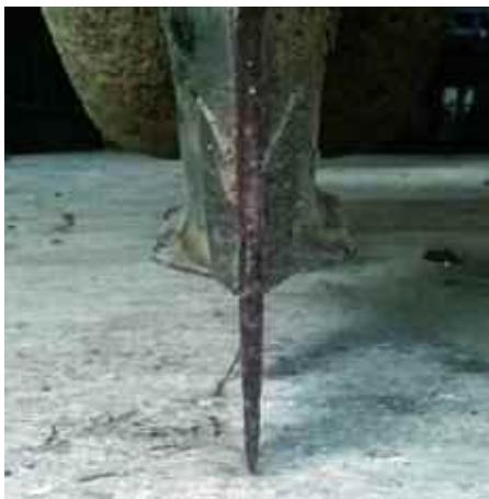
As the drill assembly slices through the soil profile it creates an inverted T-shaped slot, with seed placed on one side and fertiliser on the other.
