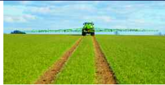
With an RTK-correction signal provided by the mobile phone network, John Deere's auto-steering system provides inch-perfect positioning pass after pass.
