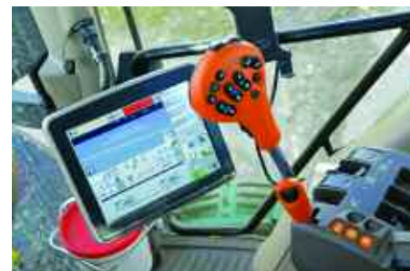
John Deere's Greenstar 2630 touchscreen terminal sorts out all the GPS functions, such as auto-steering and section control.
