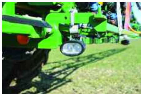
Deere's standard boom lights were swapped for an £80 pair of off-the-shelf LED spotlights.
