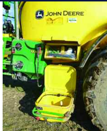
The induction hopper drops almost to floor level — great for loading with powder, but not so good for lots of repetitive filling with small cans.
