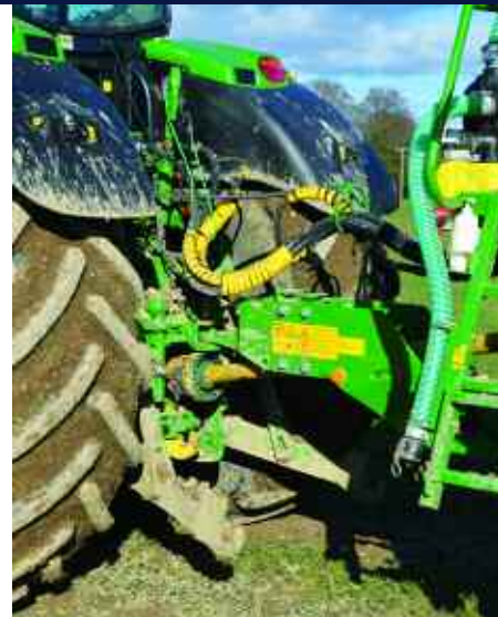
The high-level wagon hitch comes in over the top of the pto to couple with the tractor just below the top-link bracket.
