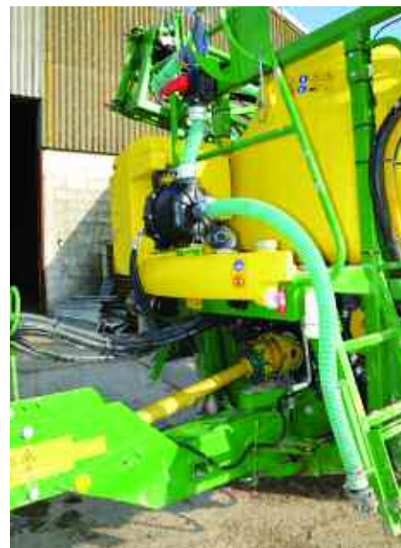
For liquid fertiliser, fitting one of Hypro's fast-fill centrifugal pumps has cut fill time from 25 mins to just six.
