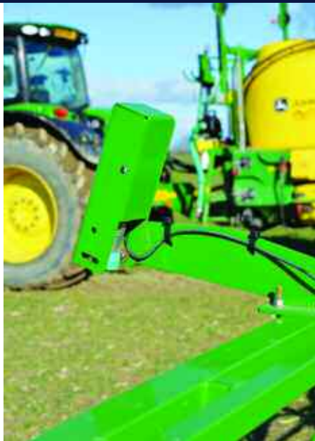
Ultra sonic sensors on the boom monitor nozzle height and lift/lower the frame accordingly – a third sensor in the centre section would improve things, reckons Will Tupper.
