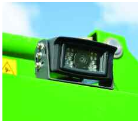
Mounted high up on the central boom frame, a bolt-on Vapormatic camera system makes backing up to trees and poles easier and travel on the road safer.
