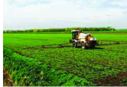
Advanced nozzle control systems allow operators to select different nozzles, from the cab, to comply with LERAPs and other restrictions.
