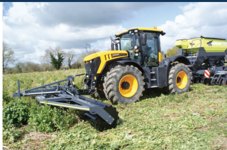
A front-mounted rolling stalk chopper helps to flatten the cover in front of the drill.
