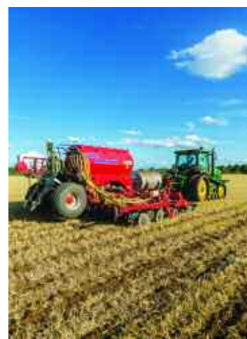
Using 'smart' technology means that drilling at a variable seed rate according to risk is possible across the whole field.
