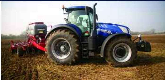
The new tractors can be fitted with some serious rubber, up to 900mm on 42in rims, which put a firm footprint of at least four lugs to the soil on each wheel. Photo courtesy Nick Barlow
