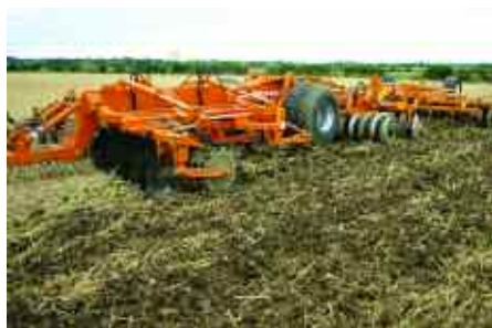
The Simba Solo So goes in straight behind the combine to cultivate the land when it's dry.
