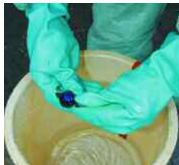
Remove the nozzles and filters and soak in a bucket containing 50ml of AllClear Extra per 10 litres of water.
