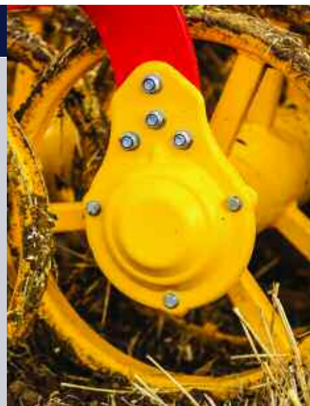
The SoilRunner roller has U profile rings designed to fill with soil to leave an open, cultivated surface.
