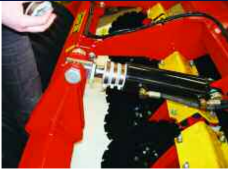
The depth is set with collars on the disc ram, so that stale seedbeds are created no deeper than 50mm.
