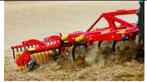
The deeper tines on the Cultus mixed the weed seeds throughout the soil profile.
