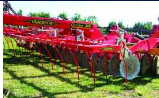
The CrossBoard on the ex-demo machine was replaced with the Straw Harrow option.
