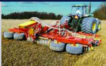
The popularity of sowing cover crops means an increasing number of Carriers are now being equipped with the firm's BioDrill.
