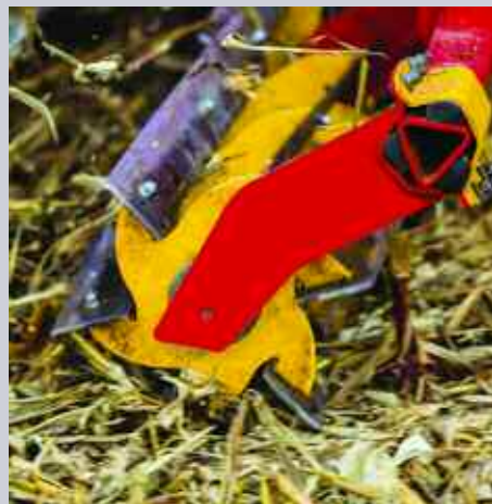
The new CrossCutter front tool aids trash break down by bashing and bruising the material.
