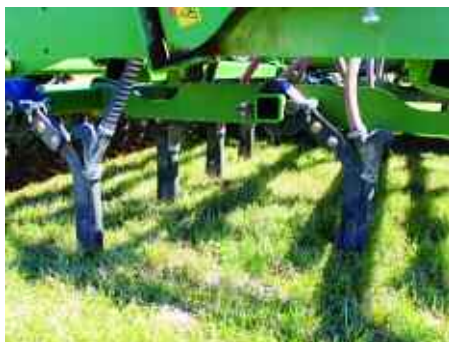
Seeder tines are rubber mounted for stone protection and to aid soil shattering.
