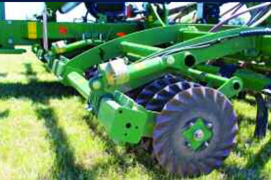
A set of wavy front discs do the initial cultivation work.
