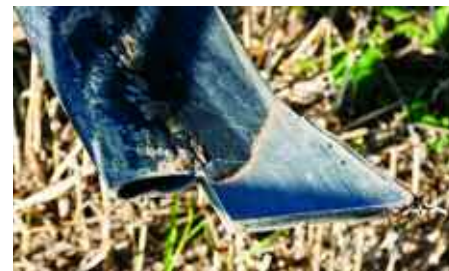
Seeder pipes can block with soil in sticky conditions.
