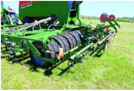
A sprung levelling harrow covers the seed before being pressed with a large-diameter rubber tyre packer.
