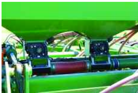
A split hopper and twin metering system allow seed and fertiliser to be applied.
