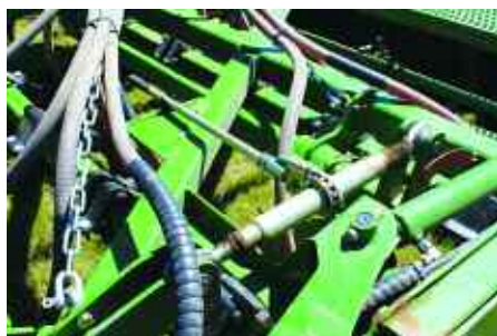
The manual depth adjustment is a bit of a fiddle until you get used to it.
