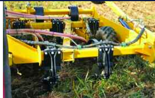
The option of new discs from Claydon will cut through the cover crop and the A-shares can be replaced with narrow tines.
