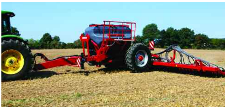
The Horsch Avatar SD direct drill uses two rows of single-disc coulters and its ability to exert a 200kg pressure on the discs to slice through high levels of trash.
