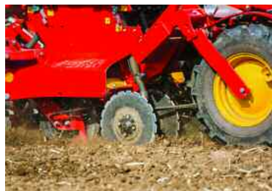
Lifting out the cultivation discs helps reduce soil disturbance on the Väderstad Rapid.
