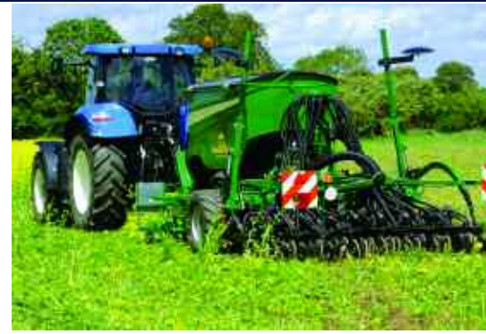
The Great Plains Saxon drill is fitted with Turbo Coulters designed specifically to reduce disturbance and cut through cover crops.
