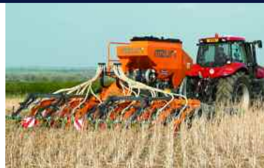
The Mzuri has a spring-loaded pivoting disc at the front to open up the soil with minimum disturbance.
