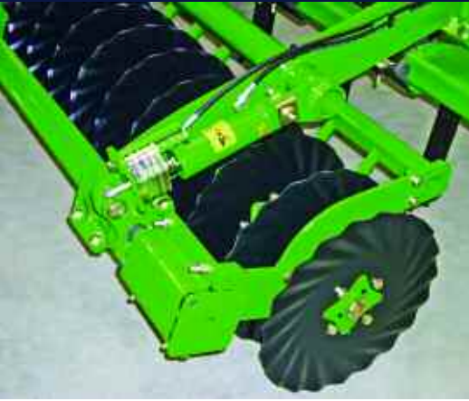
Amazone's Cayena drill is already equipped with narrow tines for minimum disturbance and now has a row of front discs for work in cover crops.
