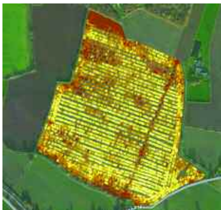
An electrical conductivity scan of the SPot Farm site shows an area of heavier soil as well as an old pipeline across the right-hand section of the field.
