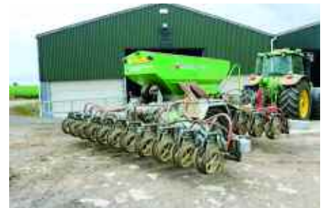
Nearly all the farm's cultivation kit was traded in to offset the cost of the new 4.8m Cross Slot drill.
