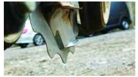
The Cross Slot pulls an L-shaped coulter through the soil, placing the seed on a shelf beside the vertical slot.
