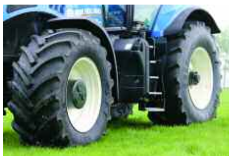
The Super Flexion Tyre (SFT) is a recent addition to the Mitas Premium range for high-horsepower tractors and harvesters.
