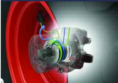
The Fendt Variogrip has an airline that runs neatly through the axle and pressures can be adjusted on the in-cab Varioterminal.
