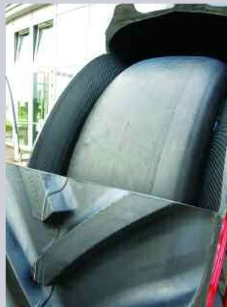
The Aircell vessel can release its high-pressure air into the rest of the tyre, boosting pressure by up to 1bar in less than 30 secs.
