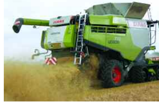
There's now the ability to dis/engage and fine-tune the chopper from the cab.
