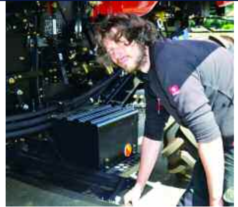
The slide-out composite trays under the clean grains and returns elevators simplify the cleaning process.
