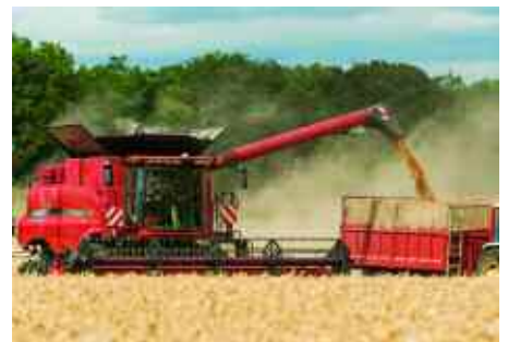
The Axial-Flow 6140 Cross Flow's separation system compensates for side slopes of up to 12°.
