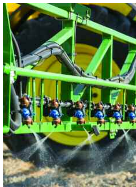
Syngenta recommends Defy 3D nozzles alternate forward and backwards, while Agrovista trials suggest forward and straight down is better.
