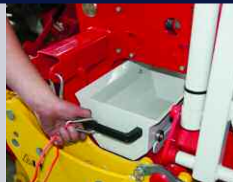
The calibration unit runs on two tracks under the metering system, and slides out, so there's no clambering under the drill.
