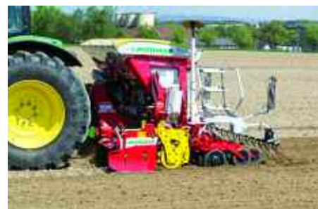
The Aerosem 1002 series seed drill is mounted over the rear roller of the leading tillage implement, such as a power harrow.
