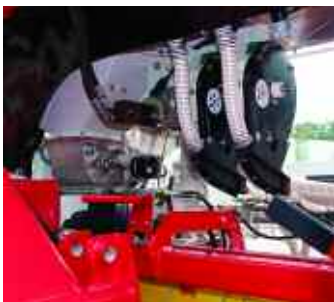
Up to 10 individual seed elements place maize at a row spacing of 37.5cm or 75cm and sit separate to the main pneumatic seed distribution head.
