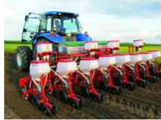
The Maga 8-row precision drill is a good choice for contractors who drill forage and biogas maize as it has variable row-width settings.
