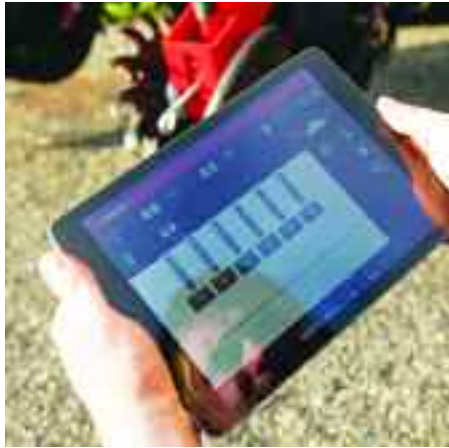
Drills controlled by ISOBUS or E-Control are also equipped with a Gateway which communicates with an iPad.
