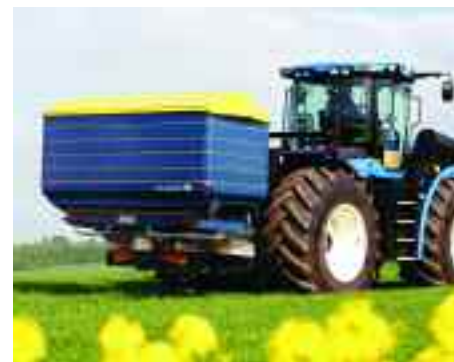
The Bogballe M6W has a hopper capacity of 6000kg and a spread width of 12-42m making it the highest capacity linkage-mounted spreader on the market.
