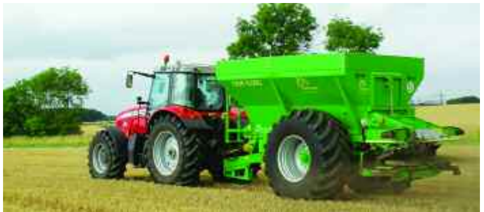
Essex based contractors R and M Simeon solved the problem of large-scale application by using a Gustrower GDK6000 trailed lime and fertiliser spreader.
