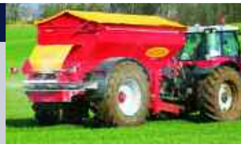
The Bredal F10 has full ISOBUS control with weigh cells together with section control and variable-rate spreading.
