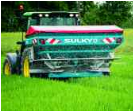
Sulky's top of the range X50 mounted spreader has a working width up to 50m and maximum hopper capacity of 4000 litres.
