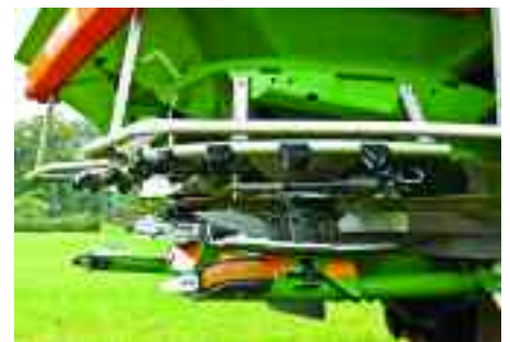
Amazone's ZA-TS series now features the optional Argus Twin spread control system, with radar sensors mounted above each disc unit to monitor the spread pattern.
