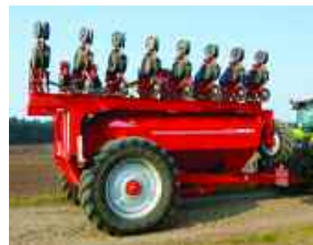
It's a big drill, but for road transport it folds to 3m when it's all shut up.
