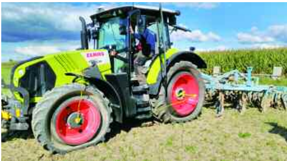
Mitas' PneuTrac tyre combines elements of rubber tracks with conventional pneumatic tyres and looks like a combination of the two.
