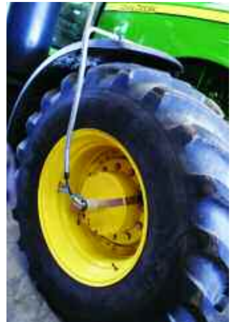
After-market inflation systems, although a great idea, have externally fitted pipework that could get damaged.
