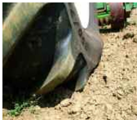
IF tyres carry 20% more weight than a standard tyre but at the same pressure, while VF tyres will carry 40% more weight at the same pressure.
