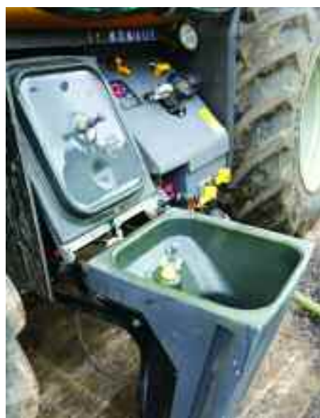
The induction bowl and controls are well set out and easy to use and the tank fills at a top speed of 800 l/min.
