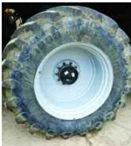
The RoGator 655c is shod with Trelleborg TM1000 710/60/38 Ultraflex tyres which provide good traction but low compaction.
