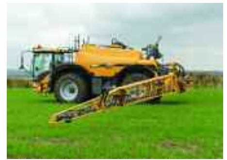
The 32m Chafer triple-fold boom is on a 24 and 32m pattern, and also has a Norac three-sensor system for ground or crop canopy sensing.
