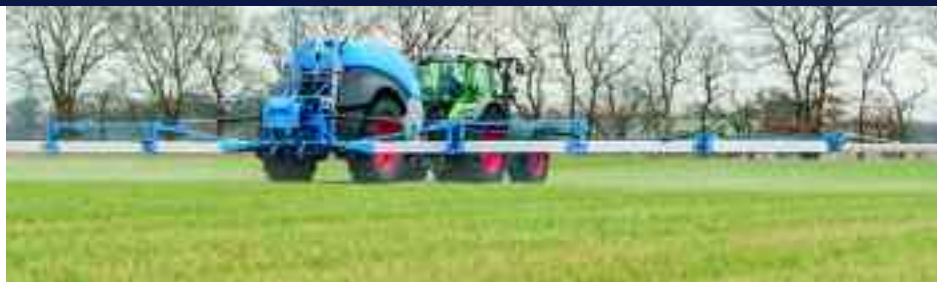
The Lemken Vega trailed sprayer is now available in boom widths of up to 30m.
