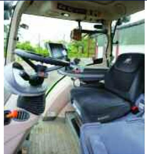
*In the cab the Varioterminal 10.4B offers touch-screen technology and controls the VarioGuide automatic steering system and Variotronic IM implement control.*
