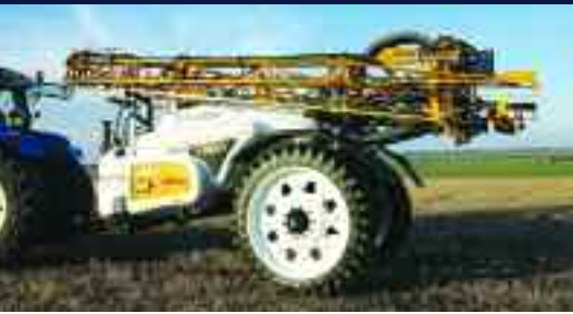
Knight Farm Machinery's new Xplorer Series 3 trailed sprayers have 3000 or 4000-litre spray tanks and steel booms of 12-28m.
