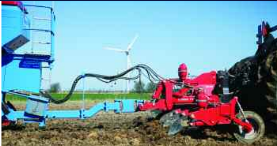
He-Va's new Combi-Lift Pre-Cultivator allows soil loosening at the same time as drilling or cultivating.
