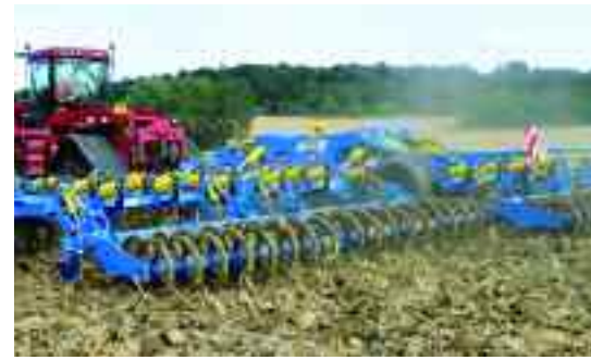
The Farnet Phantom range of heavy-duty springtines is suitable for mid to high horsepower tractors, with widths from 6-12m.
