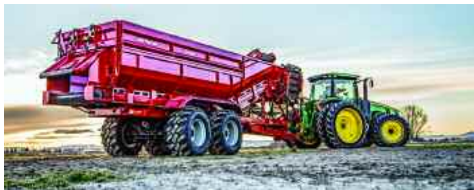
Grimme's new Crop Cart has a 20t holding capacity, handles crops gently and minimises soil compaction.
