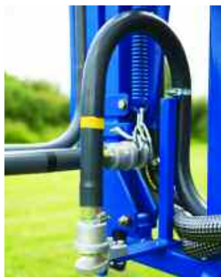
Any damaged deflector plates or poorly maintained pipework can cause striping.
