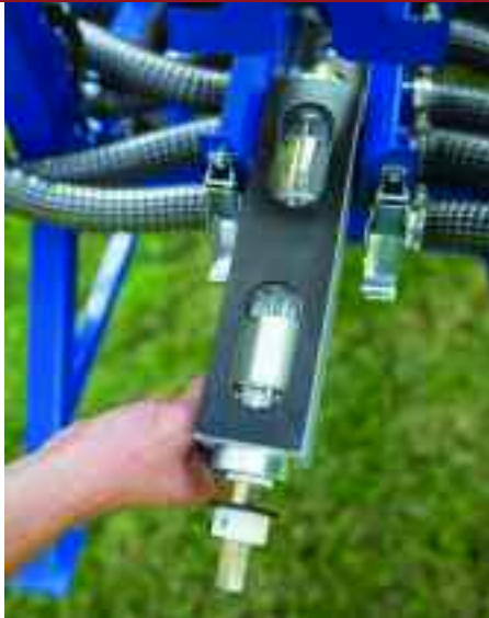
The accuracy of the TMA4 is attributed to the individual metering system.
