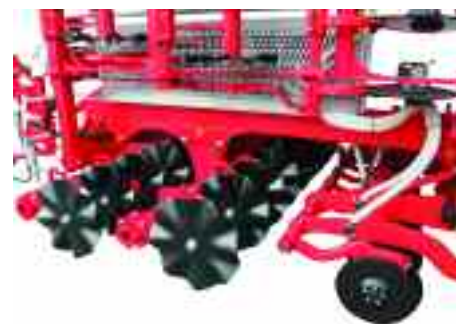
Pottinger's wave disc has a wavy profile, which is angled in the direction of travel.
