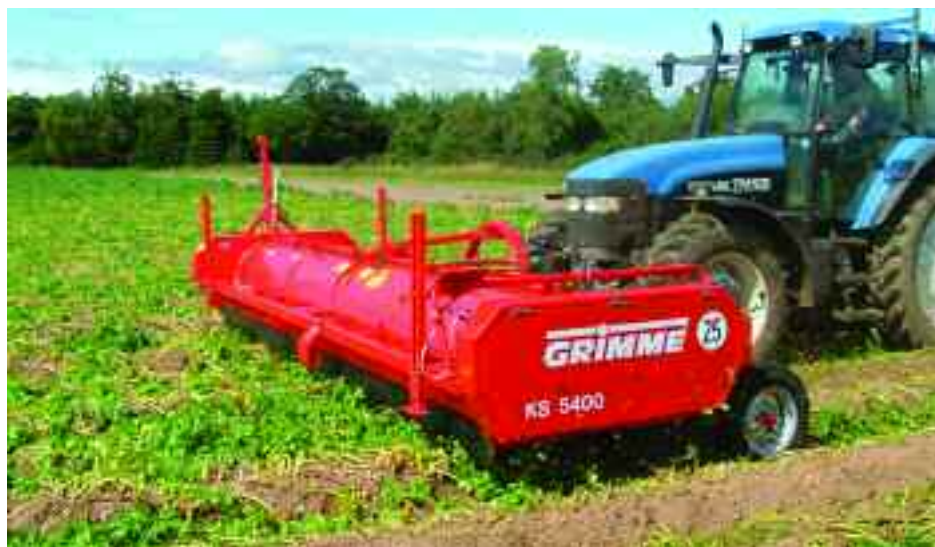
The increased number of wheelings can be a problem when flailing in a wet season, though six-row machines are available which reduce the problem.
