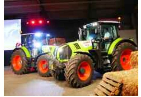
A new top-of-the-range Arion 660 will be available in 2018. Rated at 185hp, it's the only Arion power-boost model which brings output up to 205hp.
