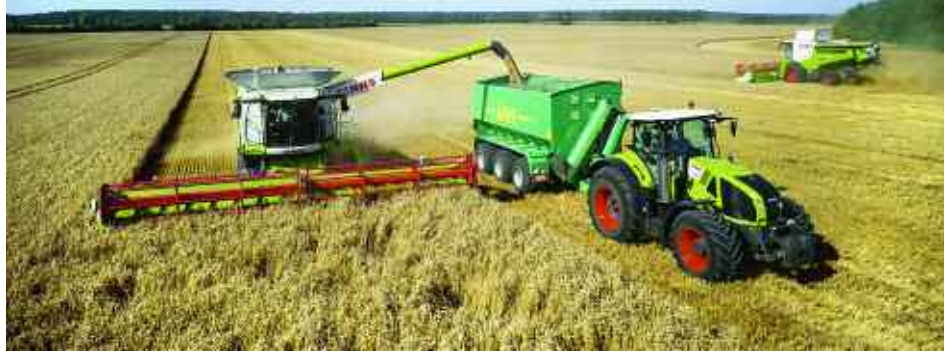
All 900 Series tractors are fitted with an updated continuously variable ZF Terramatic transmission.
