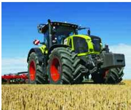
The maximum output of the new Claas Arion 920 — 960 models has been increased and now ranges from 325 to 445hp.
