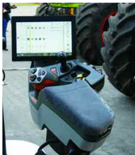
The new Cebis system has a 30cm HD colour touch screen monitor, which is available for all Arion and Axion tractors.
