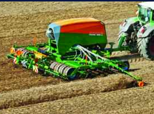
Amazone's Cayena 6001-C trailed tine seeder has a dual compartment 4000-litre seed hopper equipped with two independent, fully electric metering units.
