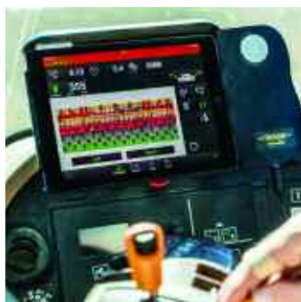
Seeding rate changes with Väderstad's in-cab E-Control system are via iPad and happen instantaneously regardless of the tractor's forward speed.
