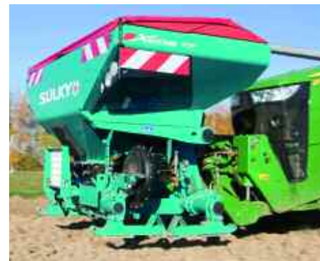
Sulky's updated XEOS TF front hopper frame allows increased capacity and better stability regardless of the drilling toolbar used.
