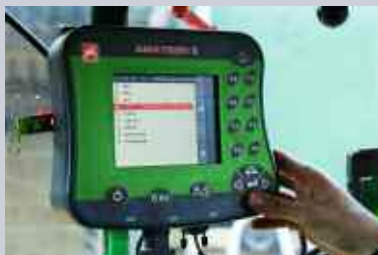
A common problem is the wrong settings on a control box — check for simple things, such as whether the sensor is turned off.
