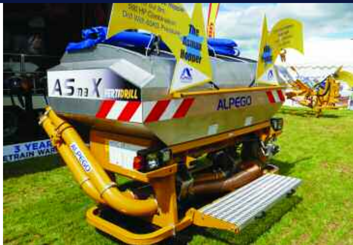
Alpego's ASMax 2300-litre twin hopper has a movable bulkhead that allows two different configurations or completely removes for seed only applications.
