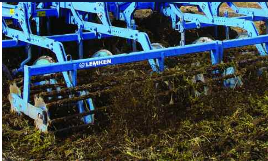
The original packer roller on the cultivator was exchanged for the tube-tooth crumbler roller that can overcome difficulties caused by the flints.
