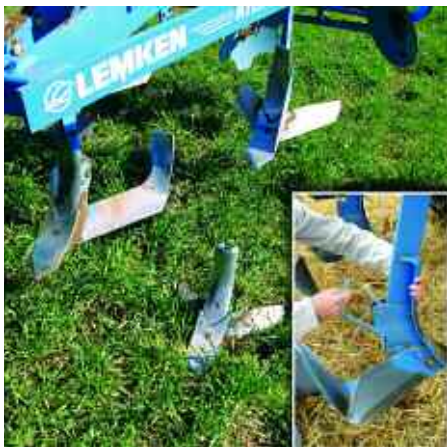
The Kristall cultivator legs offer the option of either Tri Mix wings, for maximum soil mixing, or the standard Duo Mix wing, as Mark has on his machine.
