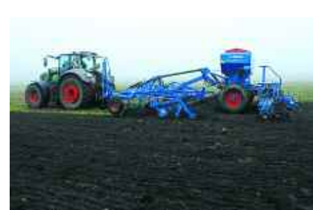
The drill can be used in tandem with a Lemken Kristall 6m cultivator, and go straight into the stubble.
