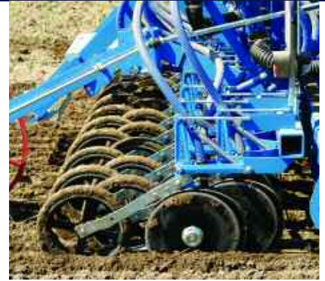
The Solitair 9 drill double disc coulters, with the parallelogram linkage that ensures optimum depth and coulters pressure.
