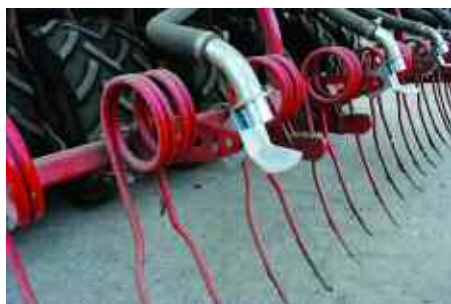
Avadex is applied through a BioDrill attached to the back of the Rapid RDA drill.
