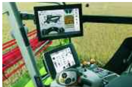
The new CEBIS Mobile 30cm colour touch screen allows the operator to adjust all the assistance system functions simply by touching the screen.
