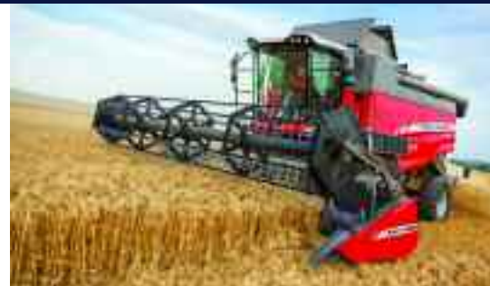
The 7345 S PL will join Massey Ferguson's range of fully self-levelling combines and will be available with the MCS threshing and separation system.
