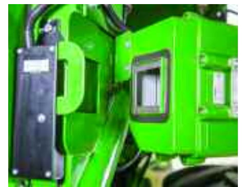
Two special cameras, mounted on the clean grains and returns elevators, monitor for cracked grain, foreign and unthreshed material.
