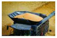
A 17,100-litre grain tank and unloading speed of 210 l/sec are among features designed to deliver a step-up in field performance and efficiency.
